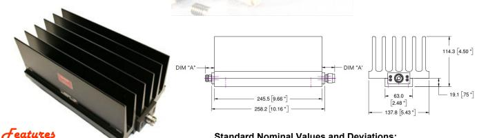
Type N, DIN 7/16 and 4.3-10 stainless steel Male/Female connectors per MIL-STD-348A. Type N connector interface dimensions mate nondestructively with MIL-PRF-39012. DIN 7/16 connector conforms to DIN 47223, IEC 169-4, VG 95250, CECC 22190. 4.3-10 connectors mate non-destructively with DIN EN 61169-54 and IEC 61169-54 interfaces. Designed to meet MIL-DTL-3933 environmental specification.
