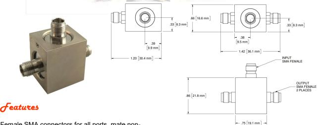
Female SMA connectors for all ports, mate nondestructively with other SMA, 2.92mm and 3.5mm connectors. Optional male connectors are available. Designed to meet MIL-DTL-3933 environmental specification.
